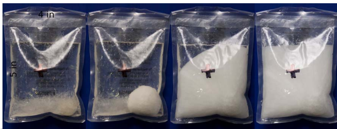
Figure 9: The crystallization of a sodium acetate hand warmer. The first picture shows the hand warmer in a liquid state, pre-activation. The second one is two seconds into the crystallization (the bulk of crystals is forming in the bottom right corner). The third picture is nine seconds into crystallization, and the pack is almost fully crystallized. The last picture shows the hand warmer completely crystallized.
